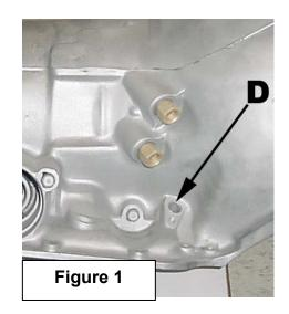
Intermediate servo spring and spring seat may be discarded. The shorter of the two spacers must be slid on to the pointed end of the apply pin. The longer spacer needs to go on the opposite end of pin and the piston on top of that. Slide the apply pin assembly into its bore. The separator plate will hold it in place. Discard all check balls.
