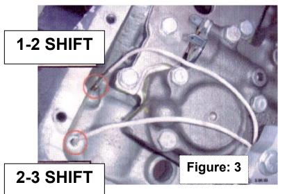
**Step 6:** Install in case the two connectors. (Figures 2 & 3)
