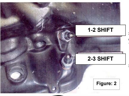
**Step 4:** Drill hole just behind cable in flat area of case with 7/16" drill enclosed. (Figures 2 & 3)
