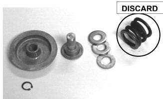
Remove spring from rear servo piston and install 3 to 4 washers to take up space.
