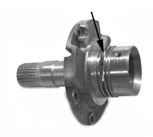
Remove spring from rear servo piston and install 3 to 4 washers to take up space.
