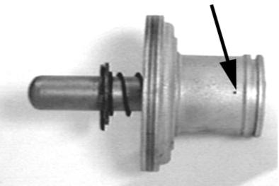
Intermediate band Adjustment; flex or hard back, tighten to 75 inch lbs. then back off 1 3/4 turns on new band or 2 turns on used band.
