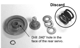
Find bleed hole located between sealing rings on kickdown servo piston (71' and up only). Drill and Tap for set screw to plug hole. Make sure it is
