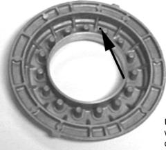
Use a 1971 and up, 4 clutch, Front Clutch Pack Drum with wide bushing (recommended or aftermarket aluminum drum should be used). The style of bushing in the drum must match the front pump support bushing area. Drill a 1/16" bleed inside the piston next to the 90-degree sealing edge between spring towers. Use a 15-spring piston; install all 15 of the 1.4 late model springs.
